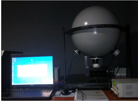
J&C TECH [ LMS200 ] : Luminous Flux
